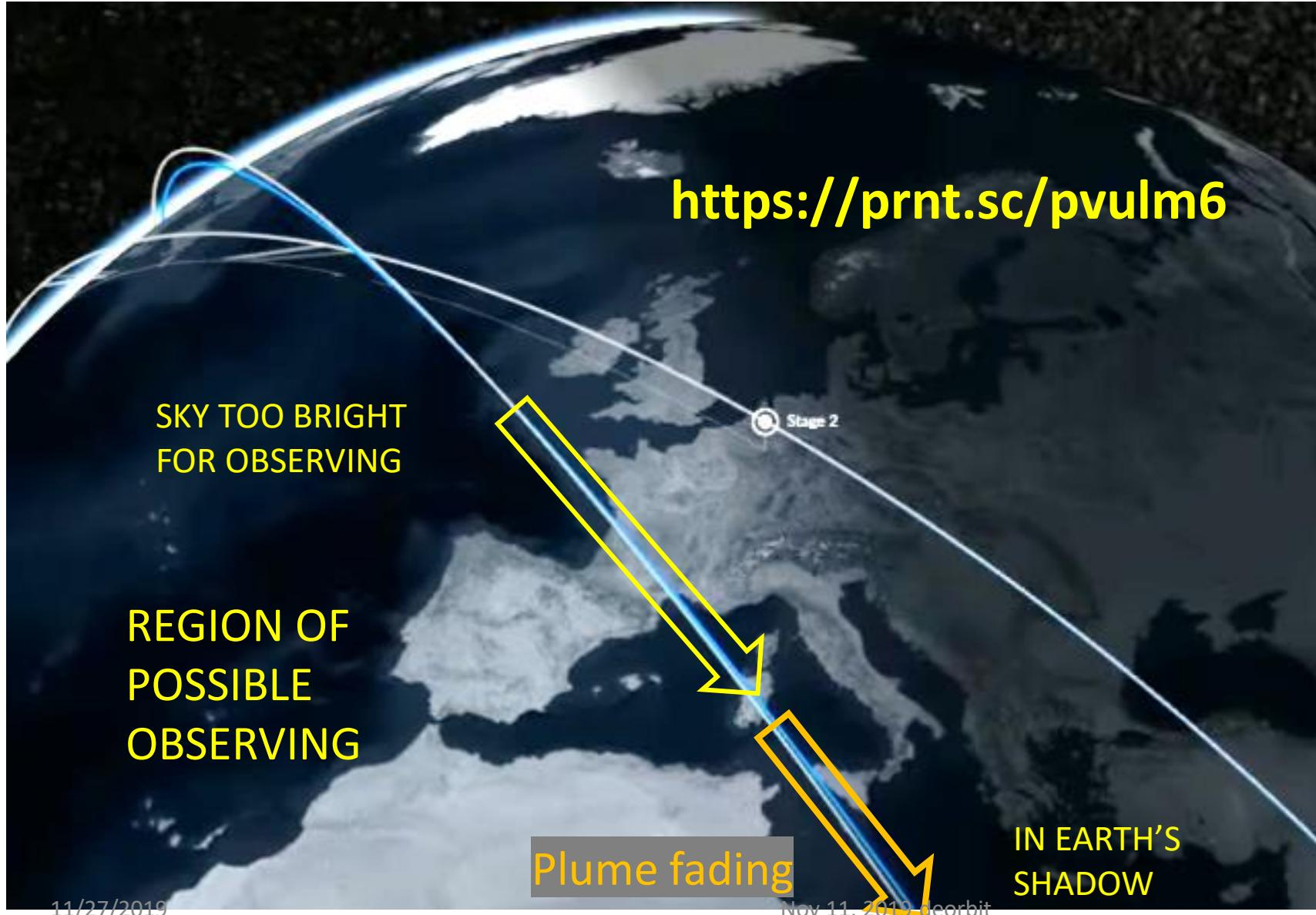
The second stage of the Falcon-9 launch vehicle made two passes across western Europe, the first while coasting [and while the sky was too bright for it to be seen]. And the second [an hour and a half later, when dark skies made it very visible] just as it made its brief braking maneuver to drop into the Indian Ocean
