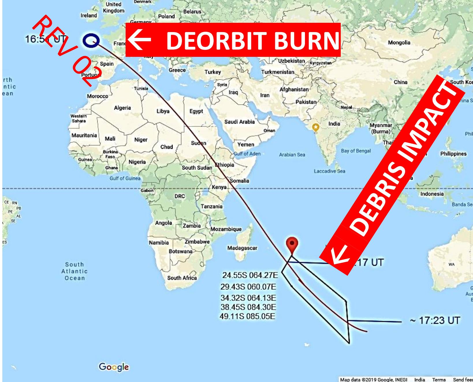
WITH REMAINING PROPELLANT, FALCON9'S SECOND STAGE TURNED TAIL-FORWARD AND IGNITED ITS ENGINE TO LOWER THE ORBITAL PATH INTO THE ATMOSPHERE OVER THE FAR SOUTHERN 'INDIAN OCEAN', WHERE IT WAS EXPECTED TO BURN UP SAFELY
